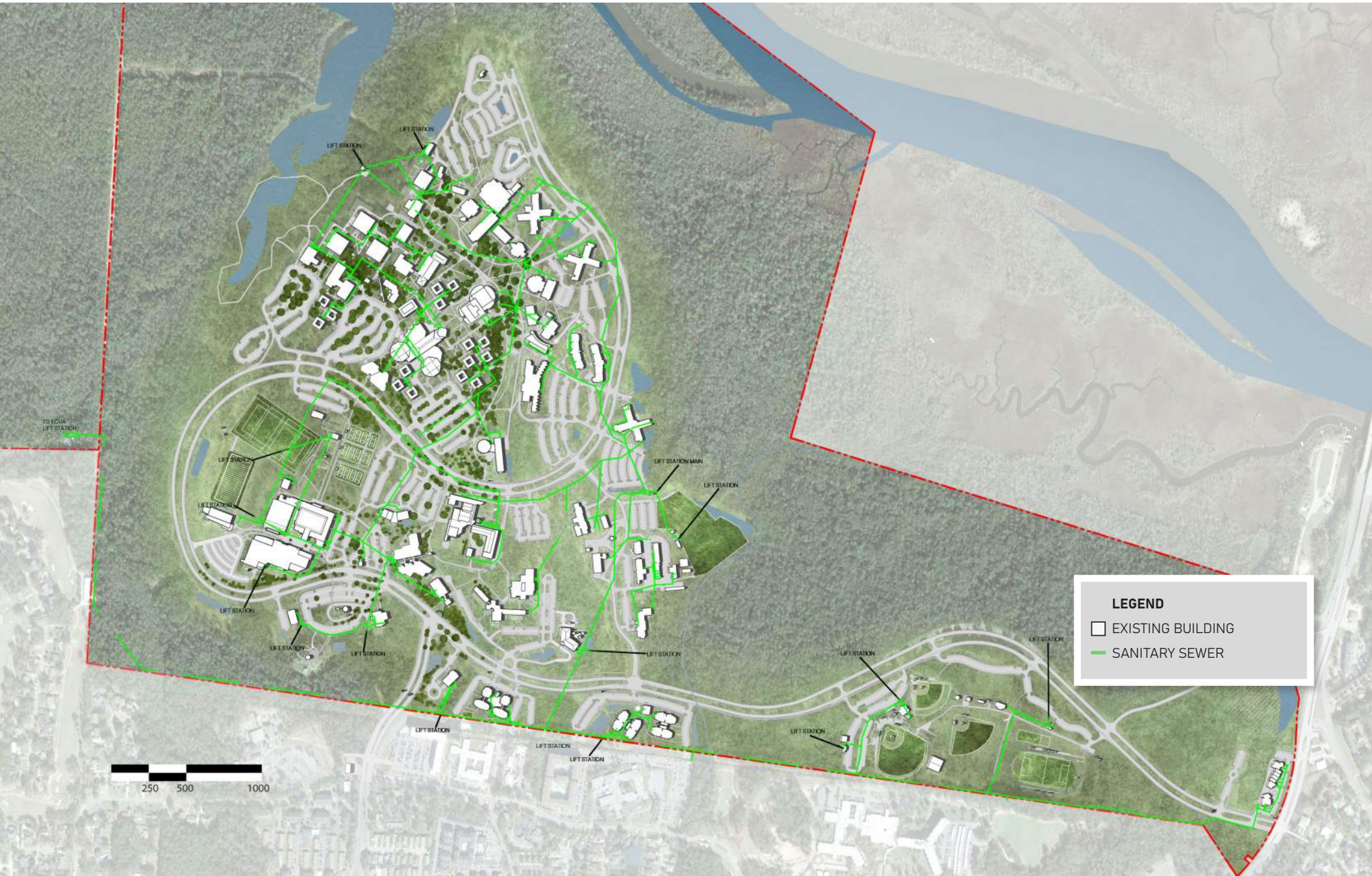
FIGURE 2.6.3: EXISTING SANITARY SEWER MAP - MAIN CAMPUS
